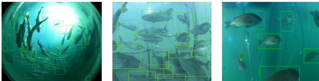
Figure 11: Example images of a fish counting system using YOLOv4 trained model. The captured video data with (left) coho salmon (middle) yellowtail (right) red seabream were fed to our fish counting pipeline, and the total number of fish in each cage was estimated automatically.
